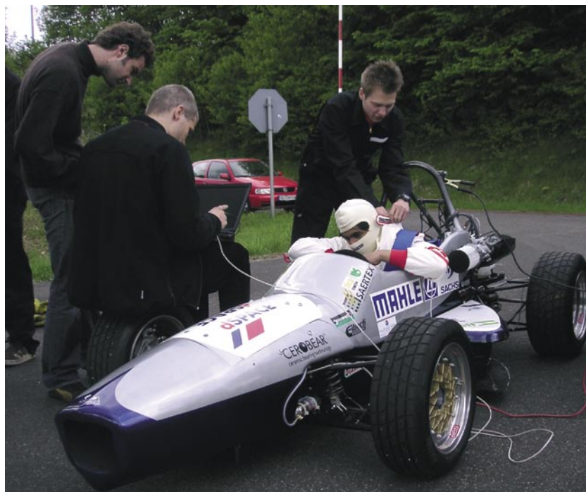
◀ During road tests, data was captured by MicroAutoBox's Flight Recorder, and later evaluated. This allowed errors in the controller model to be found.
