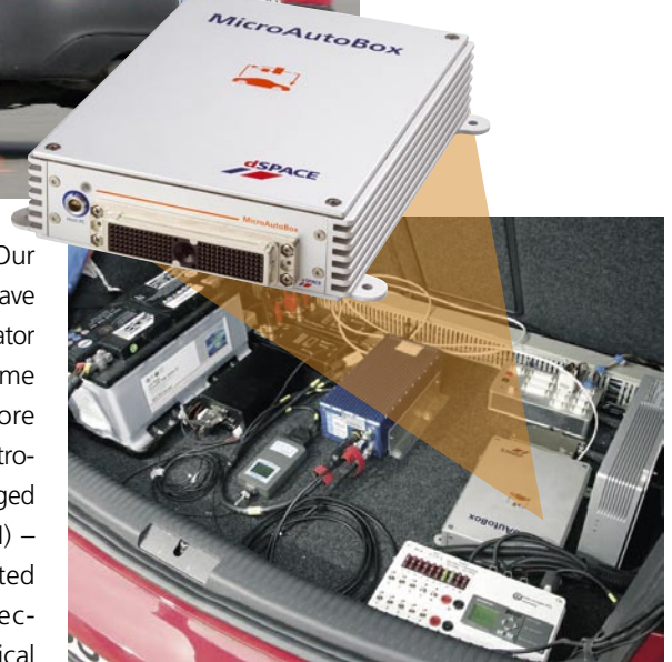
▲ The MicroAutoBox was installed in the trunk of the test vehicle.
