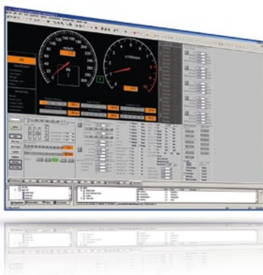
Direct control and visualization of ACC signals in ControlDesk.
