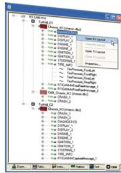
Fig. 2: The CAN Navigator is the central access point to handle CAN in ControlDesk.
