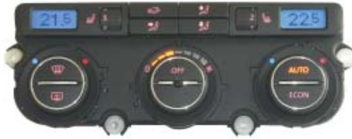
▲ Air-conditioning ECUs from Behr-Hella Thermocontrol – developed with dSPACE tools.
